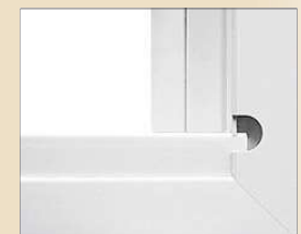
Tight, mortised-cut, double-wall sill dam extends inside the jamb, eliminating the need to caulk an open seam.
